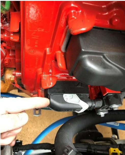
Figure 25 Cummins ECM J2 Connector
