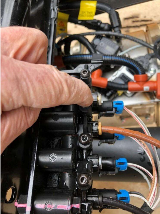
Figure 1 PTO Air Solenoid
