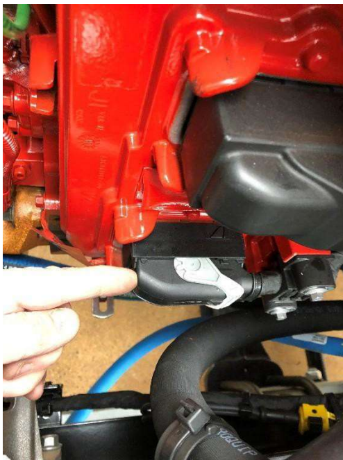
Figure 19 Cummins ECM J2 Connector
