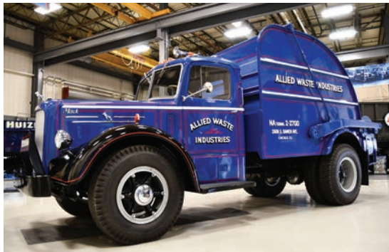
The 1952 LFTD with Heil Colecto-Pak refuse body is equipped with air brakes, a 5-speed transmission and a 6-cylinder gas engine capable of up to 158 horsepower.
