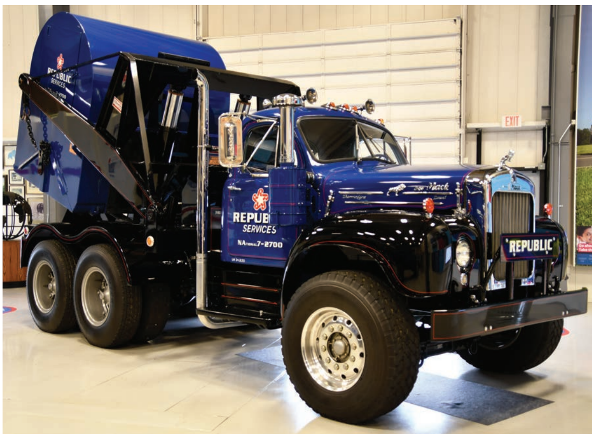
This 1965 B53S with Dempster Dumpster body has a 6-cylinder diesel engine with an 18-speed manual transmission producing up to 158 horsepower.
